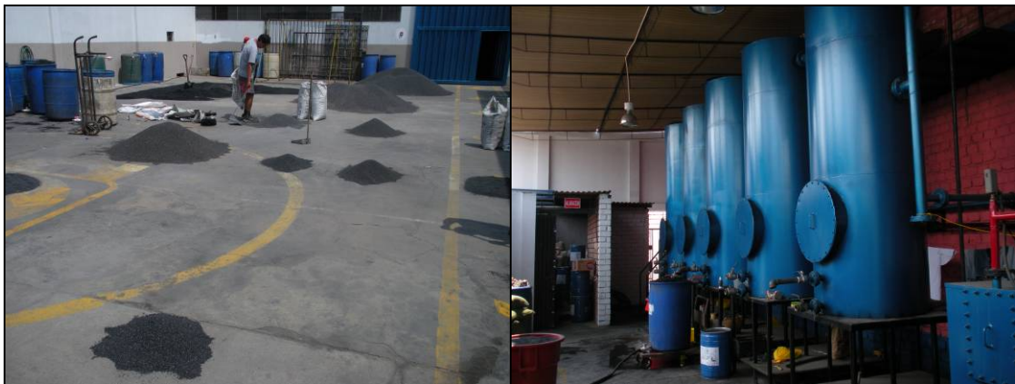
Gold impregnated activated carbon at a desorption plant, physically segregated per artisanal producer. Desorption tanks of a processing plant serving artisanal producers, where activated carbon is processed to recover the impregnated gold. Very small batches of a few kilogram of activated carbon (left picture) cannot be processed technically and economically in processing plants designed for batch jobs in the order of one ton (right picture); in case of attempting, gold losses would be extremely high and processing costs would exceed by far the benefits of Fairtrade and Fairmined certification.
